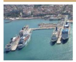
he Turkish port of Kusadasi, which comprises two piers, can accommodate between four and seven cruise ships at one time. At present, the maximum length of cruise ship accommodated is 300mtr, but this capacity will be extended in late 2004 through the construction of mooring dolphins and pier extensions.
